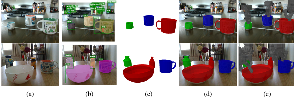
Figure 7: Grasp prediction in the wild: (a) an RGB-D (depth not shown) image, (b) open-vocabulary object detection and segmentation using Detic [43] and Segment Anything [44], (c) object meshes predicted by our method based on segmented point clouds (we filter out distant and small objects), (d) meshes projected into the original image, (e) grasps predicted by Interaction Warping projected into the original image. Figure 9 has additional examples.
